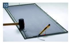
Align the fabric on the cover. Fix the fabric by using the impact keder as shown in the picture. Then cut the fabric around the keder.
