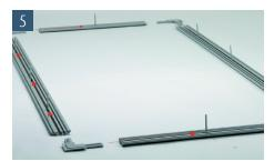
Lay out the cut profiles on a firm base. Before putting the profiles together, insert the hexagon head screws into the profile groove provided.
