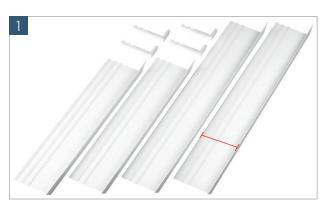
4-part insulation connection profile with corner connectors (for perimeter insulation 0 - approx. 140 mm or 0 - approx. 200 mm). The insulation connection profile can be easily adapted to the insulation thickness required on site. It must snap between 5 mm and 10 mm into the groove.
