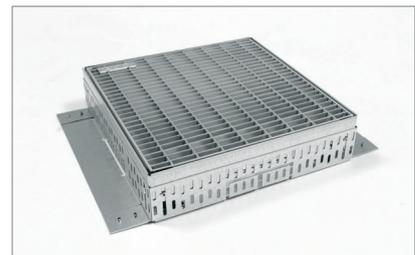
After inserting the grating, the holding clamps are screwed to the gully top through the mesh using the supplied M5 screw. Locking device of the gully tops at a fixed building height and the extension elements functions in the same way.
